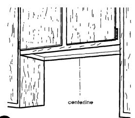
Determine and clearly mark a vertical centerline on the wall and cabinet in the area the vent opening will be made.
